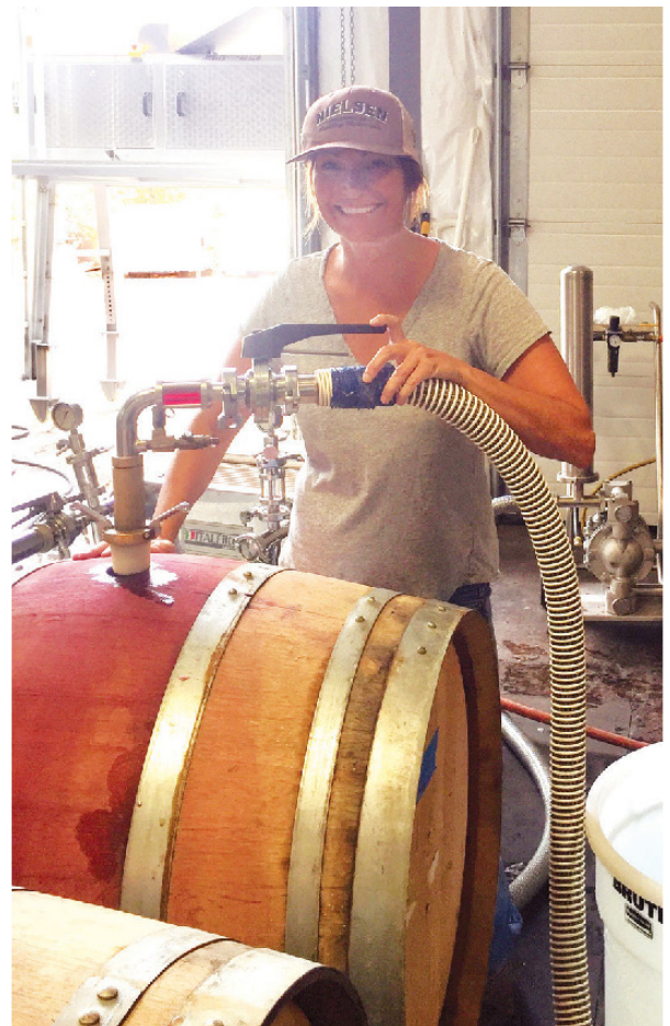
After the harvested grapes complete fermentation, the wine is moved into its first barrel. Dana's using a barrel transfer tool to transfer the new wine.
